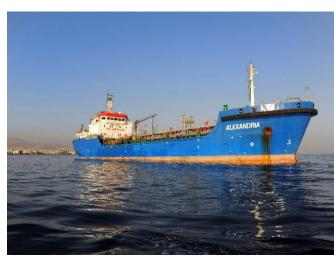
The tanker Alexandria (IMO No.: 9448889) was built in 2008, has a speed of 12.6 knots and 7,458 m<sup>3</sup> of storage capacity. The dimension of the vessel — length 94m, breadth 18m and depth 9.60m - will facilitate the permanent storage of oil-spill response equipment on board, rather than in a landbased equipment stockpile. The vessel's standard activity is shipping oil from Haifa, Israel, to Cyprus, an activity that occupies about 24 days a month of the ship's schedule.
